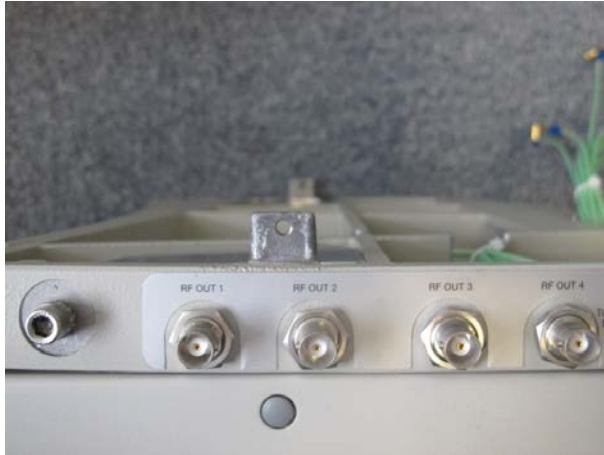
Figure 6.6: Multiple Receiver Adapter Mounted on the MAS III
