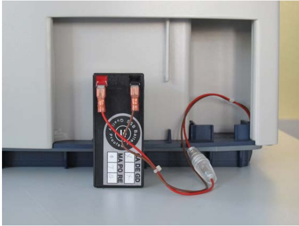
Figure 8.2: Connected accumulator with fuse
