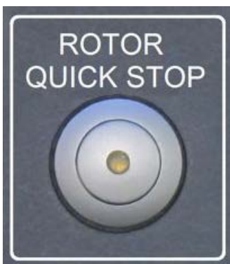
Figure 3.1: Rotor Quick Stop Button on the MAS III Back Panel
