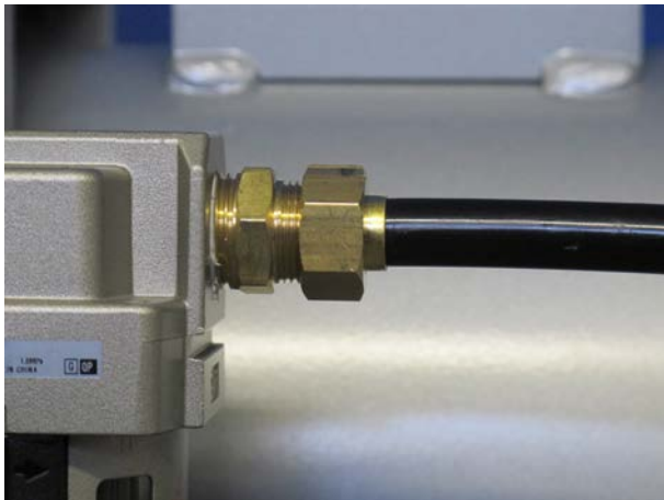
Figure 6.9: Maintenance Unit Output Connected.
