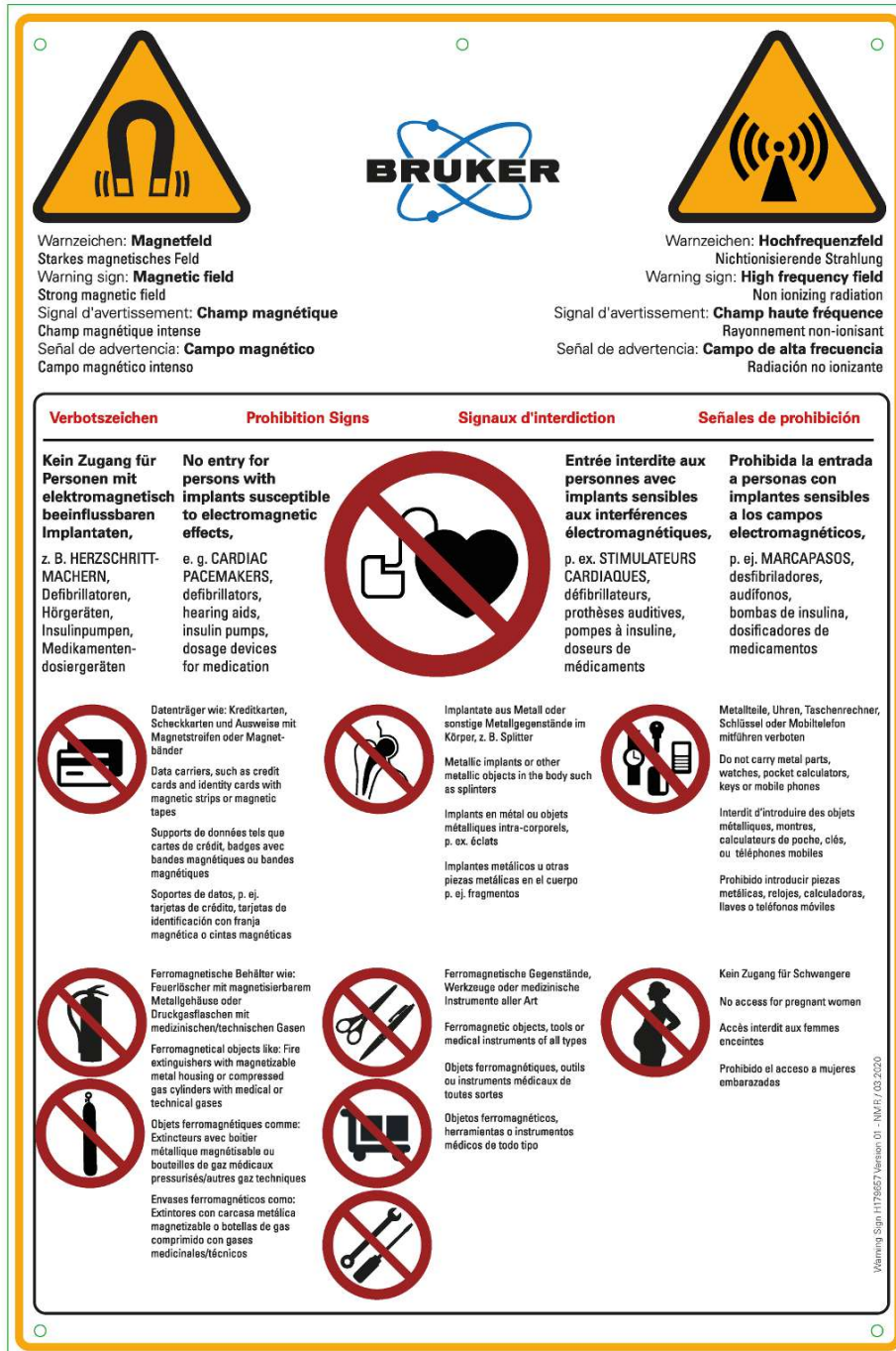
Figure 7.1: Example of a Multi-Lingual Warning Plate for Room Entrance Areas with High EMF
