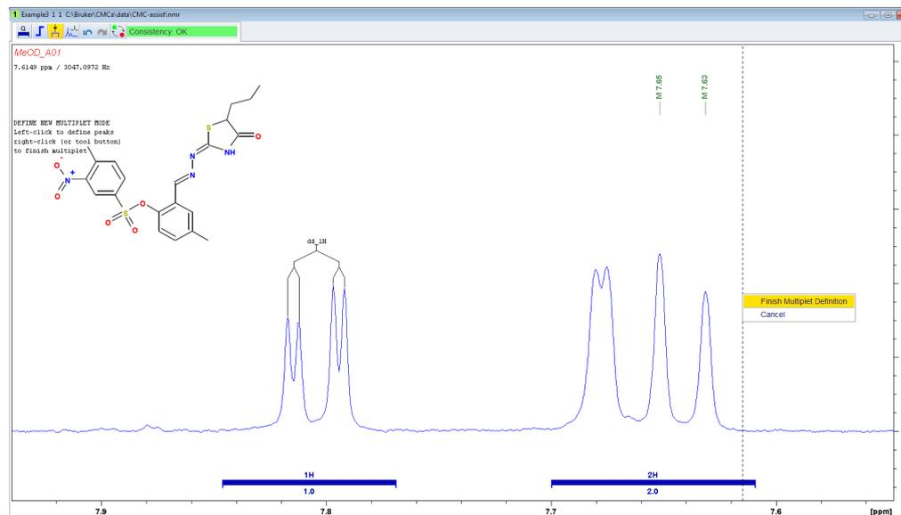
After defining this doublet the multiplet mode will be left again. The option *Redefine Multiplet* corresponds to the modification of one multiplet. For the definition of the second multiplet, right click anywhere and select *New Multiplet*. This general option allows the creation of one multiplet (exactly as described before) and afterwards also leaves the multiplet mode.
