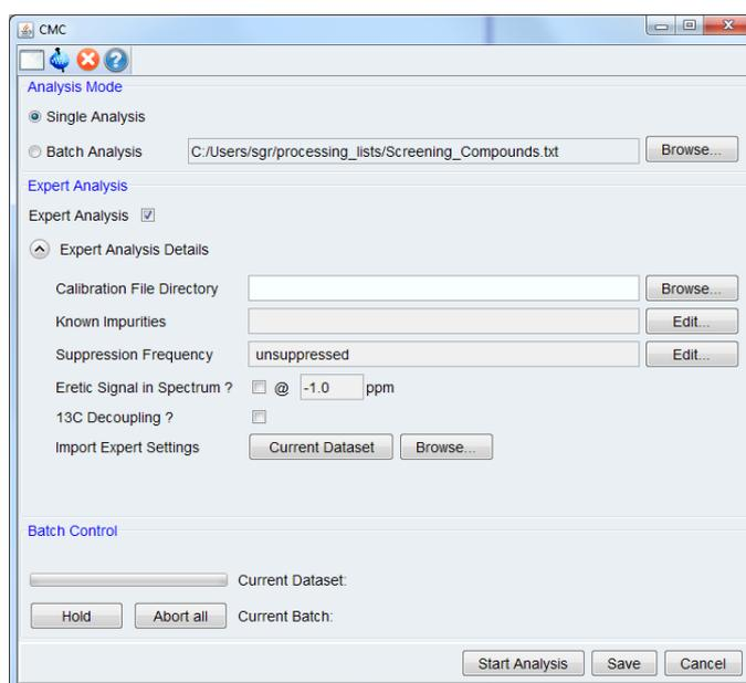
In order to reasonably analyse spectra in automation, some basic parameters need to be defined. These consist of the number of suppression frequencies, any known impurities that should be excluded from the analysis, possible  $^{13}\text{C}$  decoupling, existence of an eretic signal including its position and for quantification purposes the path to the required calibration file.
