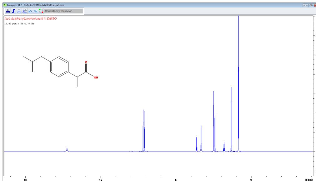
The processed spectrum is displayed together with the molecular structure and the consistency statement is defined as unknown as long as no automated spectra analysis has been performed or the statement has been modified manually. The spectrum will be analysed in automation by clicking on the tab *Analyse Spectrum* ([Analyse Spectrum](#)) which is a submenu of the *Analyse* menu.
