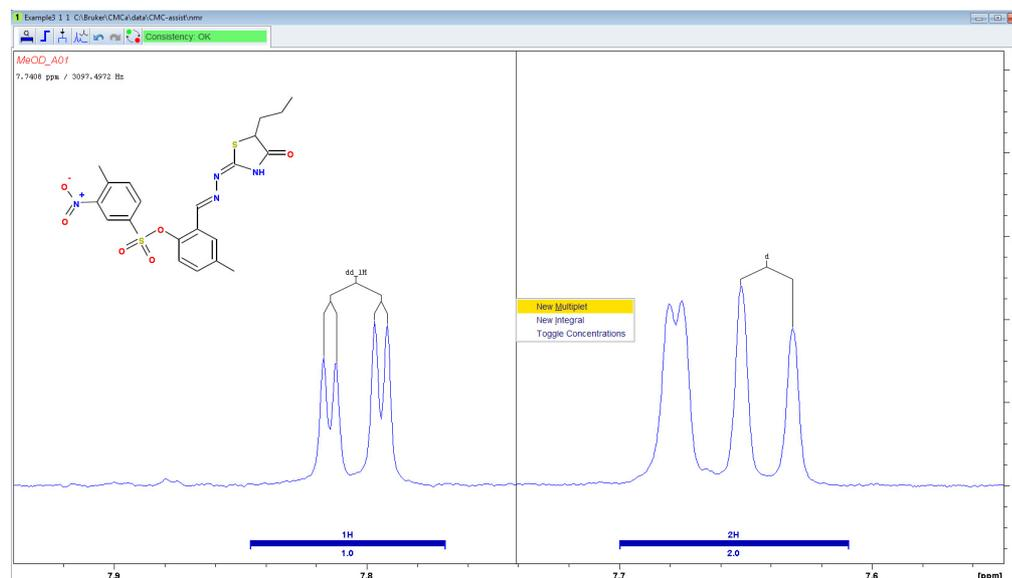
As this peak cluster consists of two multiplets now, one might want to cut the integration region and define one integral per multiplet. For any modifications on the integration
