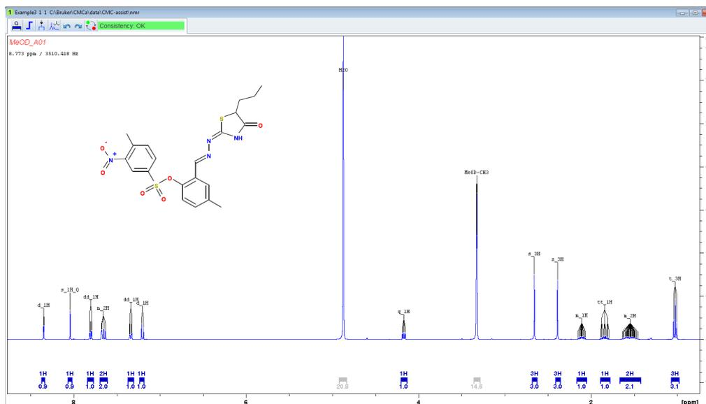
The peak cluster at around 7.66 ppm could be separated into two individual peak clusters. Therefore, the cursor line has to be close to the corresponding peak cluster with the cursor above the baseline. Right clicking offers the option *Redefine Multiplet*.
