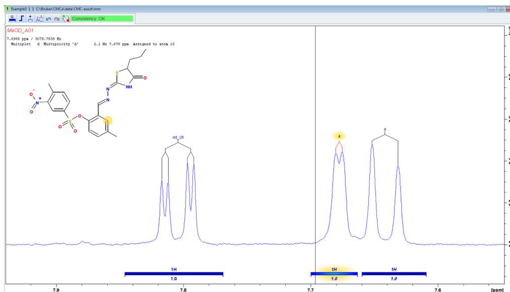
Furthermore, the automatic analysis of the peak cluster at around 4.17 ppm can be improved by manually defining the cluster as a doublet of doublet instead of a multiplet. Choose dd from the list of suggested multiplet possibilities, shown when right clicking on the multiplet and selecting the option *Multiplicity*.
