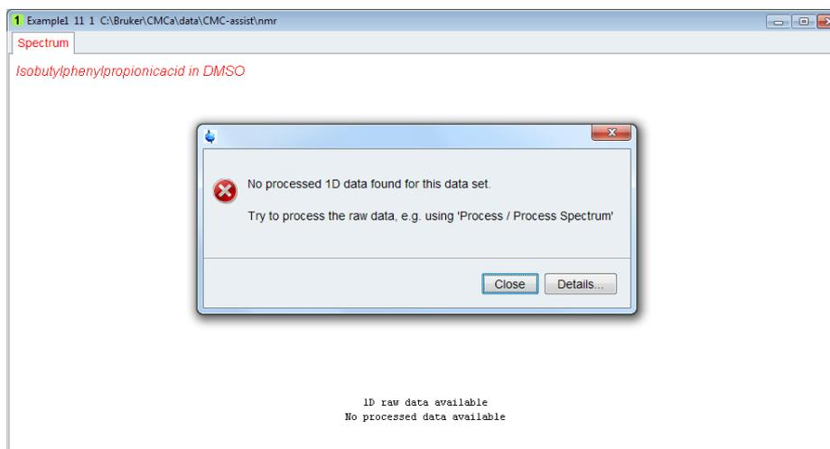
The pop up window indicates that the raw data have not been processed yet. Processing can be performed automatically using the tab *Process Spectrum* ([Process Spectrum](#)) available within the *Process* menu.
