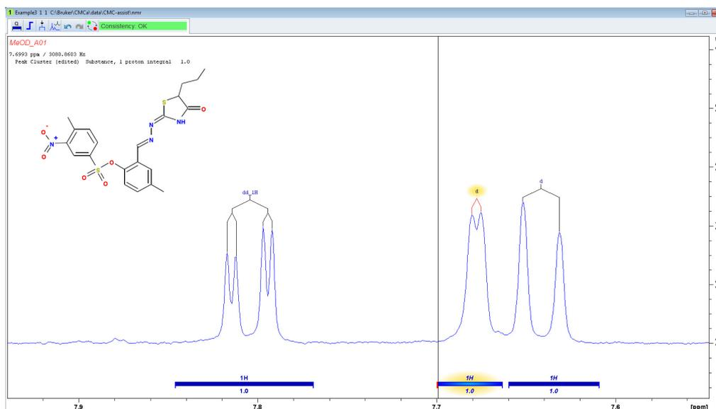
As the assignment displays the connection between the atom of the structure and the multiplet of the peak cluster, deleting the multiplet also deletes the assignment. Hence, these two redefined multiplets have to be newly assigned. In order to connect a multiplet to an atom of the molecular structure, left click on the multiplet and drag this multiplet to the appropriate atom of the displayed structure. Assignments can be viewed by moving
