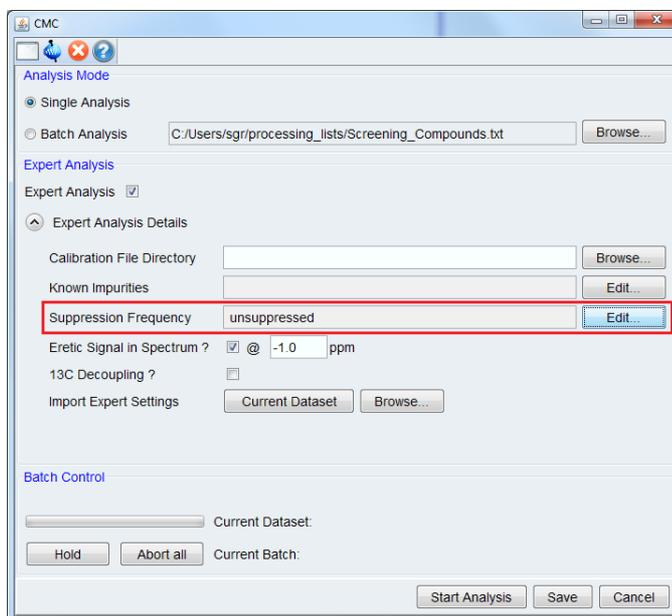
This pop up window allows modification of the number of suppression frequencies (unsuppressed, single suppressed or double suppressed) and the type of suppression (suppression frequency identical to O1P, suppression frequencies stored in a suppression frequency file or manually edited suppression frequencies).
