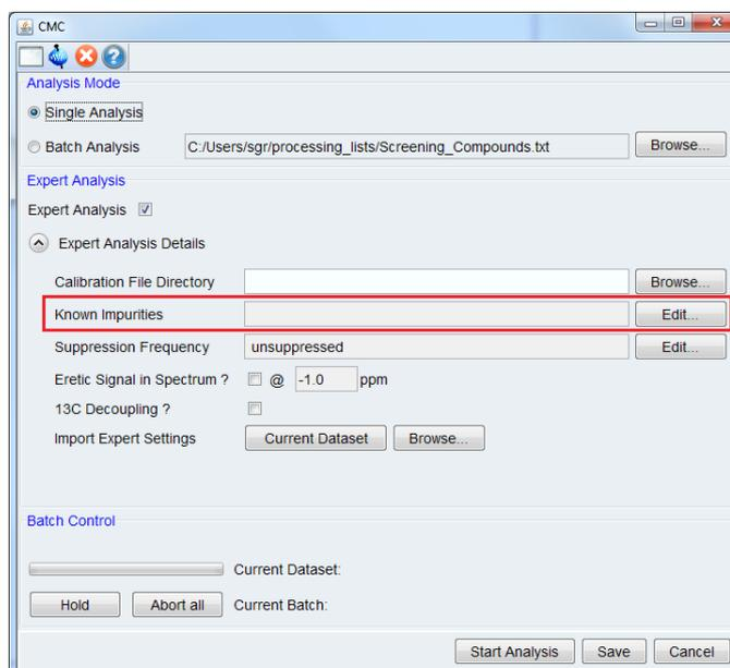
In order to define TMS as an impurity occurring in the spectrum, one has to reopen the dialog that enables modification of the required analysis information. All these settings
