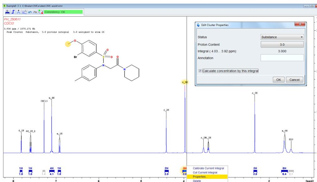
Afterwards, the down arrow on the right side of the tab *Quantification* offers the possibility to define the marked and integrated signal(s) as reference. Clicking the submenu *Define as Eretic Reference* opens up a dialog, where the assigned proton number for each labeled and integrated signal has to be entered as well as the exact concentration of the reference substance (all the given information will be saved in a file called eretic).
