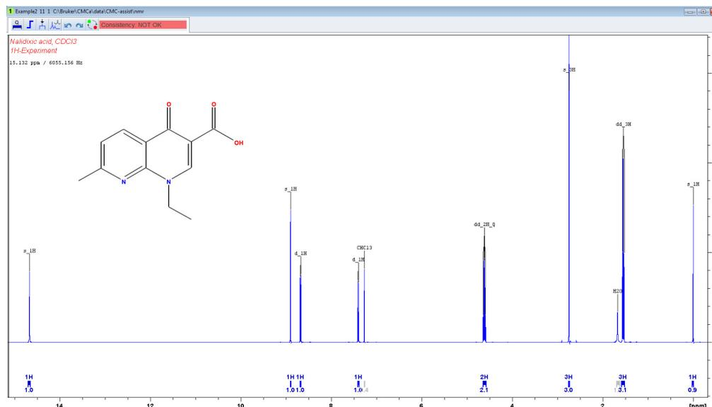
Although the software comes to the conclusion that the spectrum is not consistent with the provided structure, the spectrum gets analysed with respect to integration regions, plausible number of protons for these integration ranges, multiplet interpretation, and recognition of solvent peaks.
